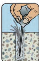
Clean drilled hole
